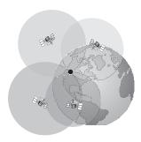
The orbits of these satellites were designed so that at any time, at any location on Earth, a GPS receiver can see four satellites. Each satellite transmits encoded information indicating its location at a precise time. The receiver uses this information to calculate distances from the satellites. Each distance then becomes the radius of a sphere, and the intersection of the spheres gives the specific location of the receiver.
